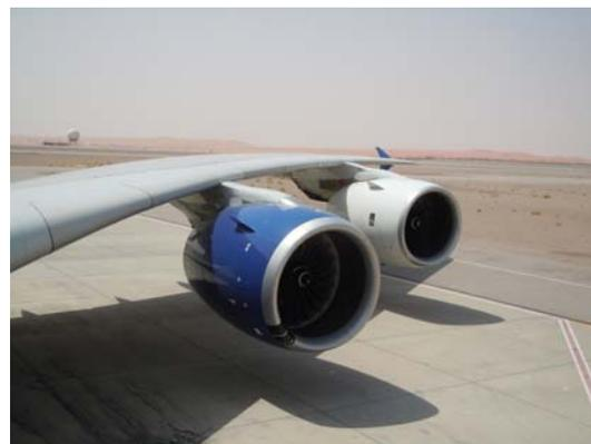
First flown in February of this year, we have completed 125 hours of flight testing with 2 development versions of the Trent XWB. Testing to date has been very successful, and it was time to stress the engine to the upper limit of external temperature. The current mid-day temperature in Al Ain, United Arab Emirates, is 44C, or about 112F. Combined with low humidity, it was exactly the environment we were searching for.
