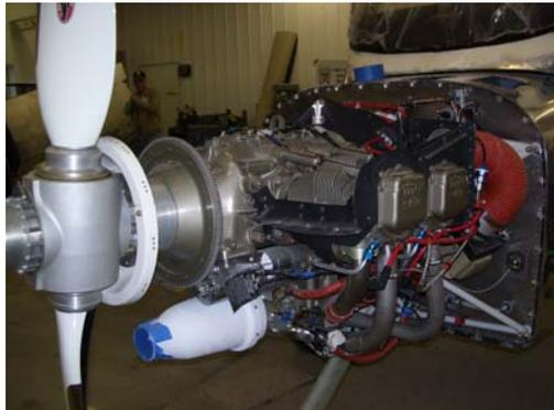
It has an Aerosport Power IO-375 engine (an increased-stroke version of parallel-valve Lycoming IO-360 engine) and a Whirlwind Aviation 200RV composite prop.
