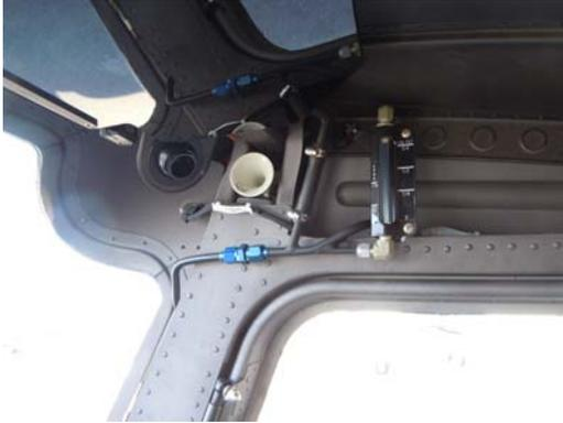
interior trim, and no carpeting. You can see all the fuel lines and control linkages behind and below the instrument panel. Fuel indication consists of sight gauges in the
