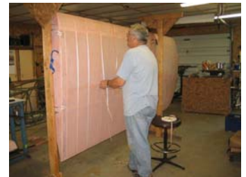
Wing #1 fabric covering & rib stitching begin ...
