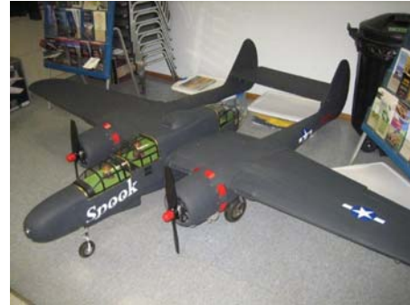
This is a Northrop P-61 "Black Widow". It is a plans built plane with small chain saw or weed whip motors.
