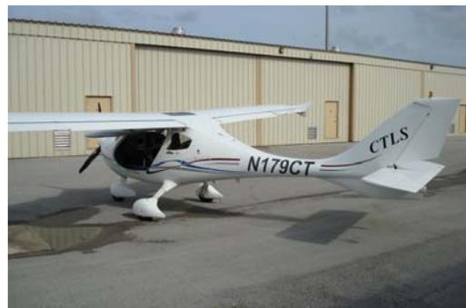
One of Brian's instructors, Chris Benaiges, was available to provide the check out. With a wingspan of 28 ft 2 inches, it fits easily in most T-hangars with room to spare. But more important than span are the aerodynamics of the wing itself. Wing area is 107 sq ft (7.29:1 aspect ratio), and the flaps
