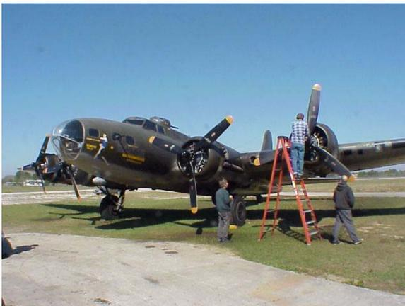
The last of the three rebuilt engines had been run up and the oil pressure was adjusted, as was the propeller.
