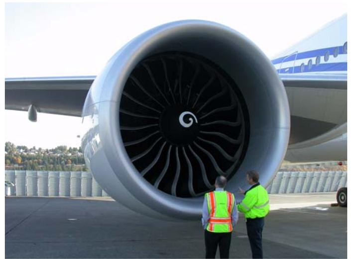
GE90-115B (115,000 lbs thrust) engine with 3D aerodynamics in the carbon fiber fan blades. The engine nacelle diameter is the same as that of a B737.
